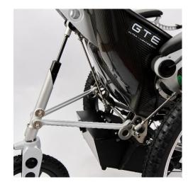
The GTE's power is delivered directly from two 24V 120W motors in the front wheels delivering speeds of up to 6 km/h, making it perfect for use on pavements or any other type of terrain. The GTE now includes a Lithium Ion battery with a range of up to 30km that's also safe to travel with by air.
