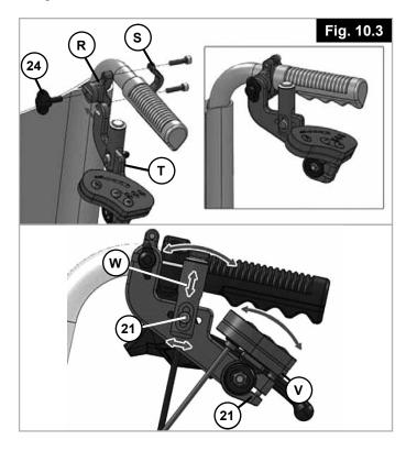
By undoing the wing bolt (24), the control unit (T) can be fully removed and stored in the back pack. To do this, pull the control unit (T) through the rear zip fastening of the back pack and store it in the right back pack pocket.
