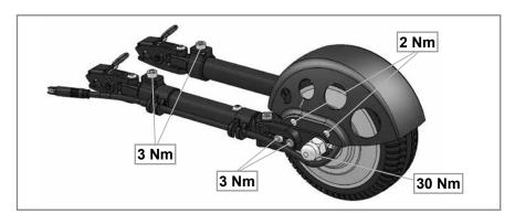
The screws used are fitted with threadlock at the factory and after fitting, cannot be re-used. After that they should be replaced or alternatively re-secured with threadlock to medium tightness.
