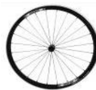
Rear wheel, Proton, 24 spokes, straight spokes
