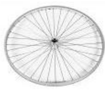
Rear wheel, Design, 36 spokes, straight spokes
