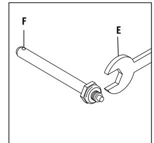
Moving the axles FORWARD shifts more of the rider's weight onto the REAR wheels, providing the following benefits: the front end of the wheelchair becomes lighter, thus reducing the turning effort, and with a shorter wheelbase the turning radius is reduced.
