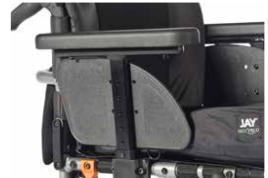
Lightweight height adjustable single post armrest Provides easy transfer and good arm support with a low transport weight.
