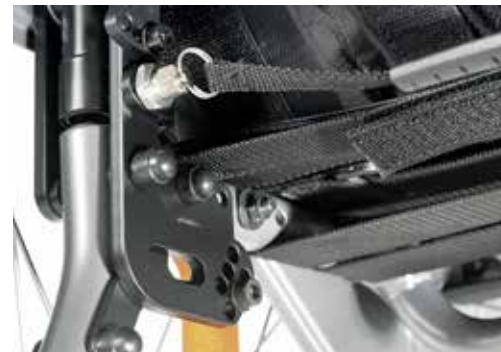
Angle adjustable back (optional) Lightweight and simple to adjust. Provides 20° of angle adjustment from -12° to +8° in 4° increments.
