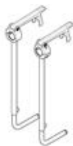
// EMF010032 Kickstand: mounted to the sub-frame
